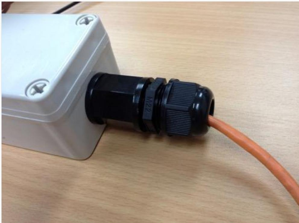
Now that we have that, we just need to insert the contracting gland to seal the Ethernet passthrough. Your stainless steel temperature sensor should now look similar to the following image.
