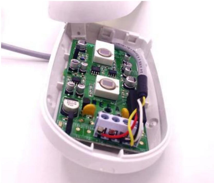
Once opened you should see 4 screws where you can connect the wires.
