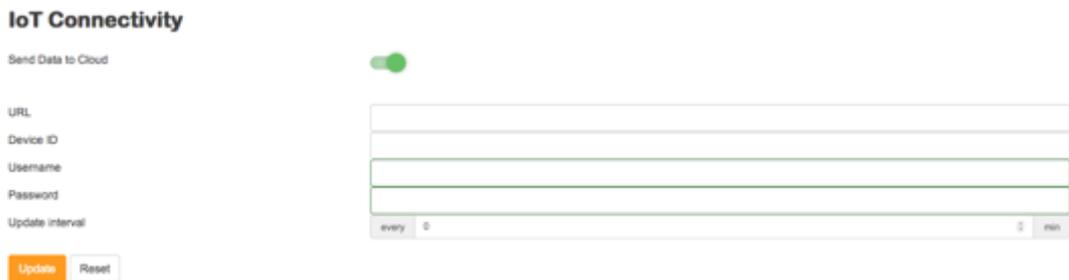
You can now input the URL where the data should go, the Device ID that will identify the gateway sending the data, Username and password for security and the update interval.
