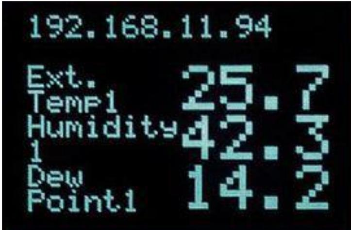
The OLED display gives one a quick view of the values the SensorGateway reading. The reference for the order of the subscript numbering is completely dependent on how the web page is showing it.
