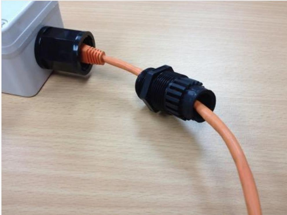
After that, connect them both on the RJ 45 connector of the sensor.
