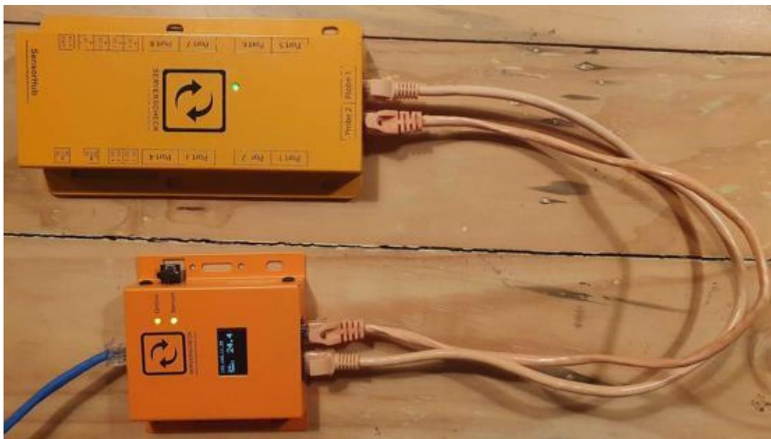
The sensor hub connects through regular RJ45 cables to the SensorGateway. The connection from the base unit going to the SensorHub should not exceed 1 meter / 3.3 ft.
