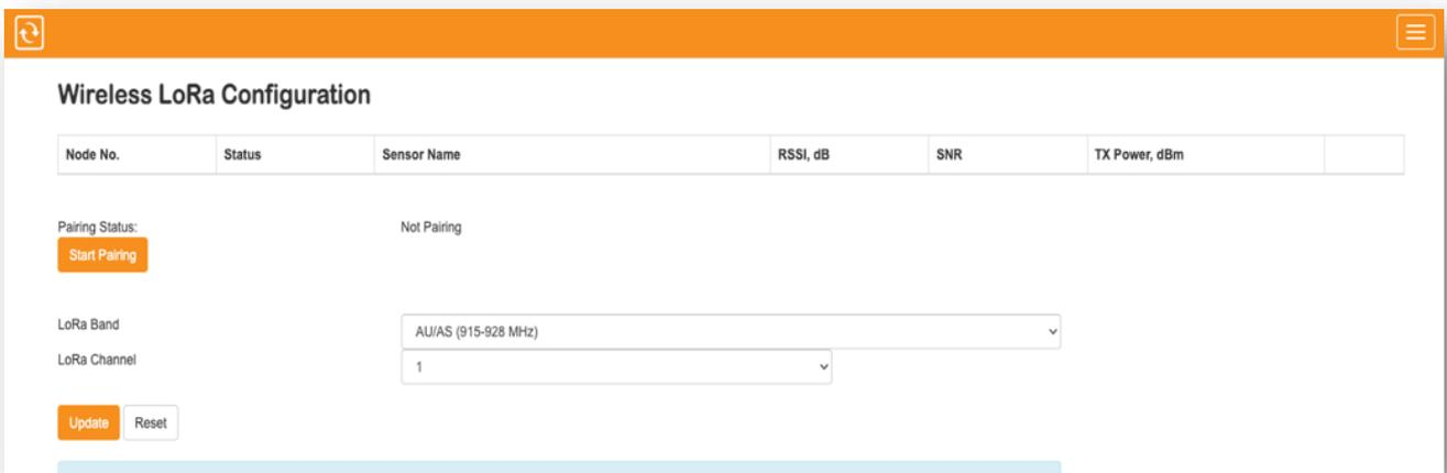
The screenshot shows the 'Wireless LoRa Configuration' page. It includes a table with columns for Node No., Status, Sensor Name, RSSI, dB, SNR, and TX Power, dBm. Below the table, there is a 'Pairing Status' section showing 'Not Pairing' and a 'Start Pairing' button. The 'LoRa Band' is set to 'AU/AS (915-928 MHz)' and the 'LoRa Channel' is set to '1'. There are 'Update' and 'Reset' buttons at the bottom.
