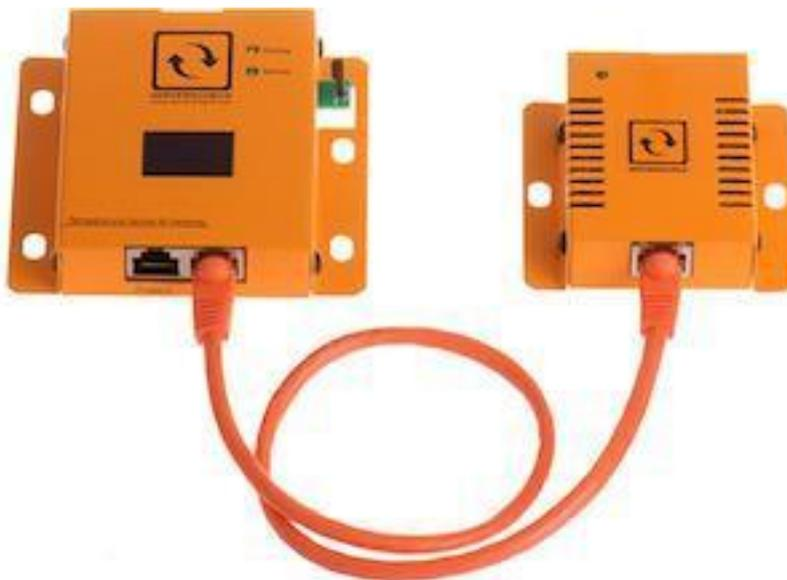
On the top you plug in your network cable connected to a switch and this into the RJ45 connector labeled **LAN/PoE**. If you don't have a PoE enabled network, then you will need the optional 12DC power adapter and plug it into the connector on top labeled **DC 12V**.
