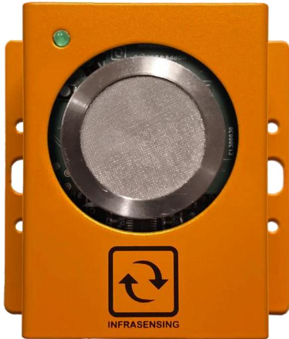
Measures refrigerant (R-134a) in the air between 0-2000 ppm (parts per millions)
