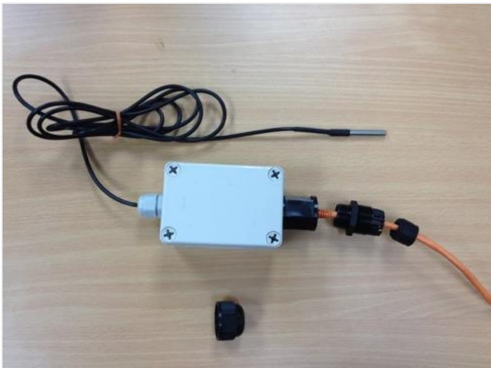
Once that's done, insert the rubber gasket all the way inside the over-nut.
