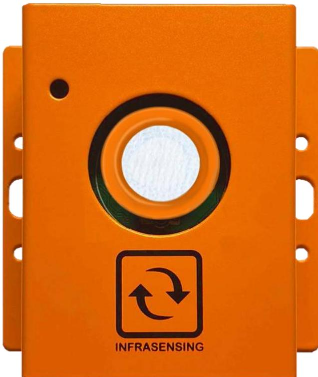
Measures Nitric Oxide in the air between 0 to 250 ppm (parts per million)
