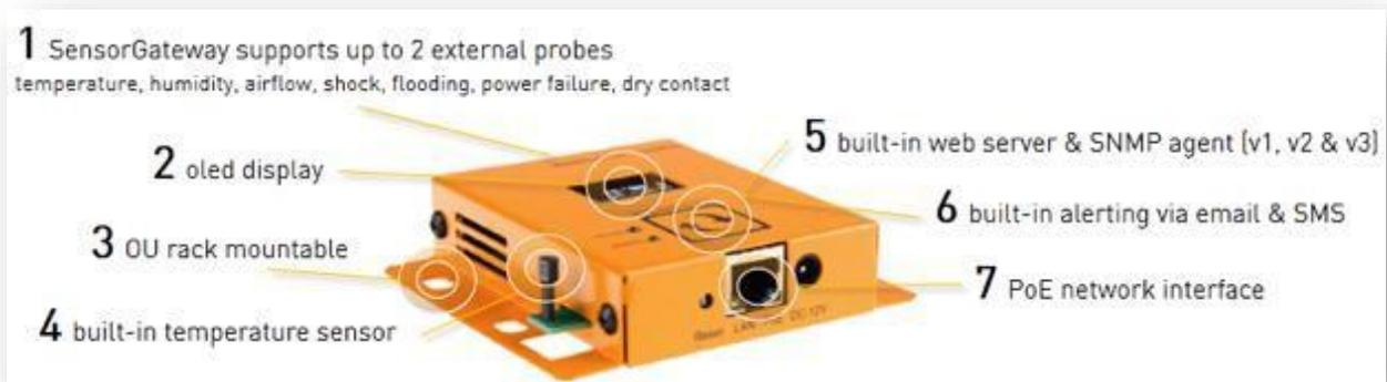
The SensorGateway is connected to the network via a standard network cable over a 10/100Mbps network. It supports PoE too. This allows for powering the sensors without having to rely on external power adapters. If you don't have a PoE network then a power adapter is optionally available.
