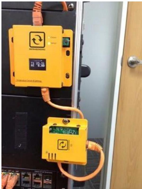
As we're utilizing floor cooling on this example, the side where the air should flow is placed facing downwards to detect the airflow it should have.
